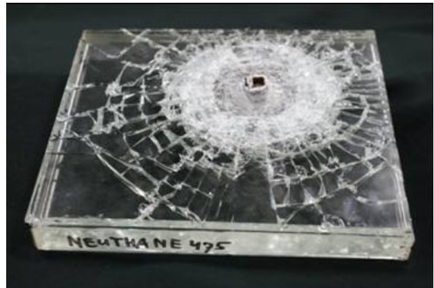
Fig. 1 Photograph of a glass-clad polyurethane after bullet impact
